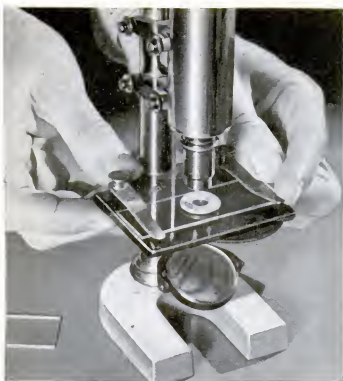
A substitute for a hollow-ground slide can be made by cementing a brass washer to a standard slide
